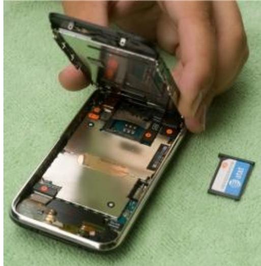
Lift the panel up from the dock end being careful not to tear or break any ribbons connected near the other end.
