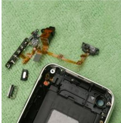
Remove the headphone jack and attached flex cable.
