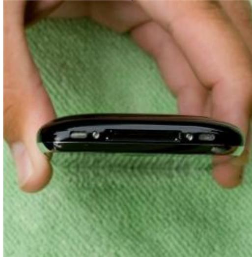
Holding your device on end you will notice two small screws on either side of the dock. These screws must be removed in order to open the case.
