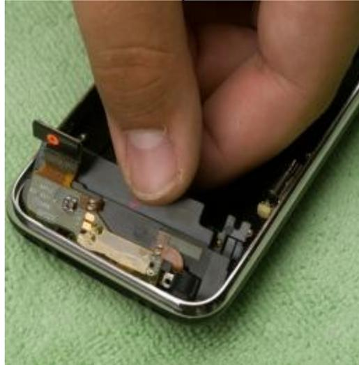
Remove the speaker assembly which also contains the dock connector, antennae and home button as well.
