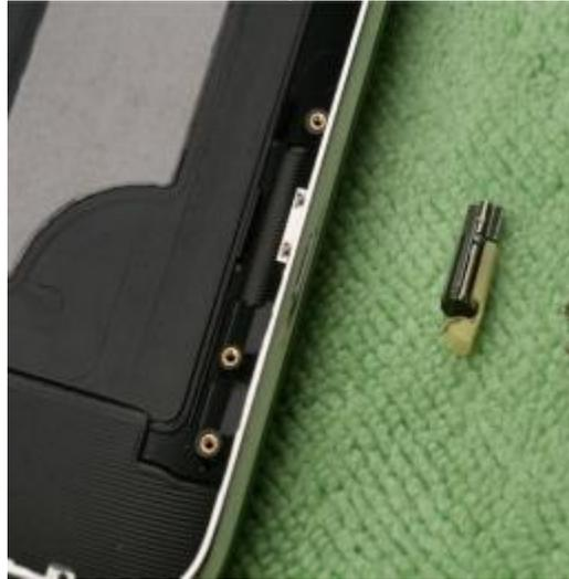
Place the vibrator assembly to the side.
