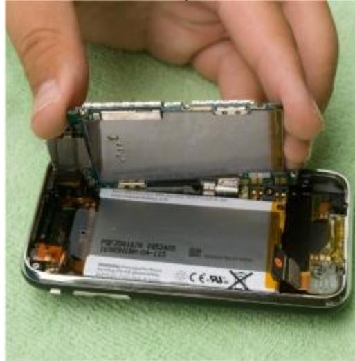
Lift the mother board out taking note of the camera which is still connected to the underside of the board. You will need to unplug the ribbon circled in red.
