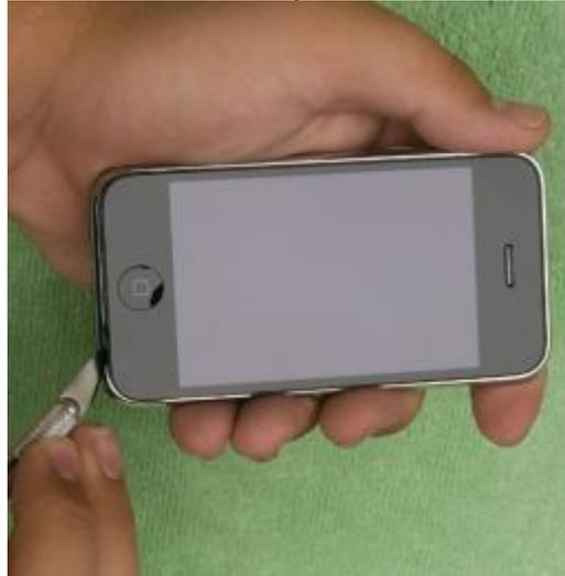
Insert a small thin tool between the chrome ring and front panel glass directly above one of the screw holes. You will need to exert a small amount of pressure to separate the display from the back panel.
