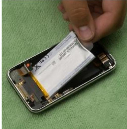
Use the attached tab to pull up on the battery, there is a mild adhesive on the back side, so it will take a bit of force.
