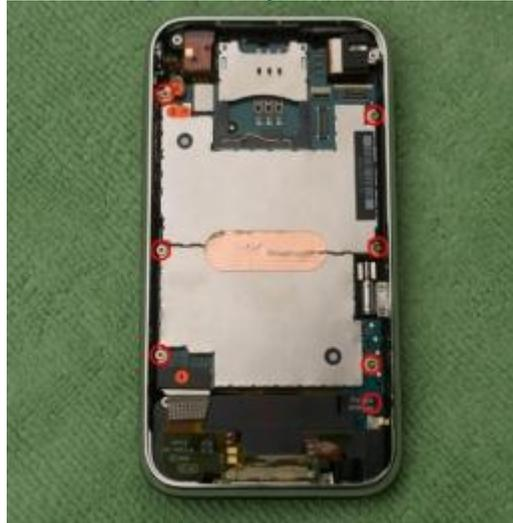
Remove the seven screws circled in red. Note: One screw is located under the DO NOT REMOVE sticker :)
